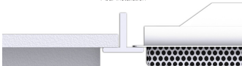
Extended Face T-bar installation
